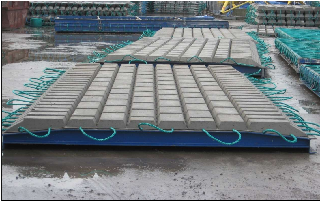
Figure 7: Example of Articulated Concrete Mattress
